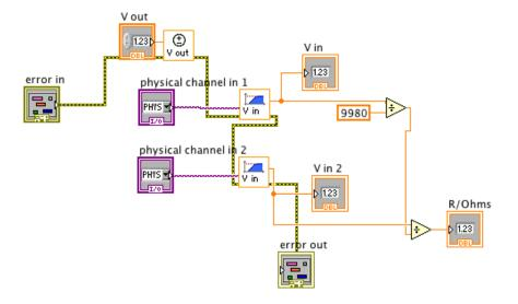
Wire the error control and indicators to the terminal block for the VI.
