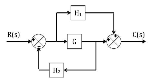
2. Simplify the block diagram shown in figure below. Obtain the transfer function relating C(s) and R(s)
