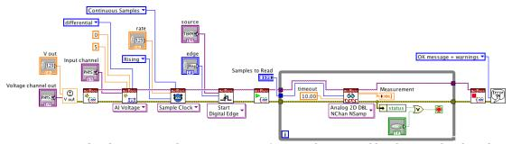
In the above circuit the source is Dev1/PFI0 and generated by shorting this digital input to ground. This starts the data acquisition. You should set up the circuit and verify this behaviour.
