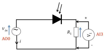
2. Use the following Basic light sensor VI and verify that the measured light intensity behaves as you expect when the light intensity is changed by shielding the photodiode with your hand.
