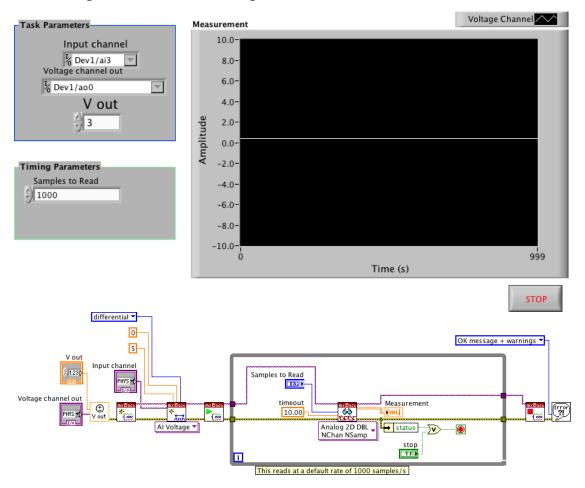
The circuit uses the default timing of 1000/samples per sec. The size of the buffer is given by the "samples to read" control. Convert the previous VI to this new form and investigate the performance.
