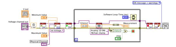
In this circuit the data is collected one sample at a time. At a predetermined time after this the next sample is read. (n.b. The minimum and maximum value of the input data should be set to 0 and 5 V respectively. The display may need to be set to "Autoscale-y".)
