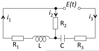
$$\frac{dI_{1}}{dt} + \frac{R_{2}}{L} \frac{dQ}{dt} = \left(\frac{R_{1} - R_{2}}{L}\right) I_{1}; \quad I_{1}(0) = I_{0}$$
