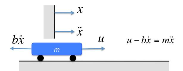
•Define the position and velocity of the car to be the state variables  $x_1$  and  $x_2$
