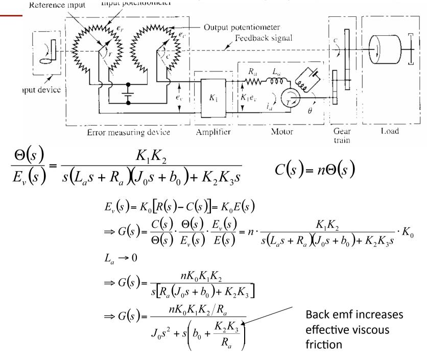
$$\Rightarrow G(s) = \frac{nK_0K_1K_2/R_a}{J_0s^2 + s\left(b_0 + \frac{K_2K_3}{R_a}\right)}$$
